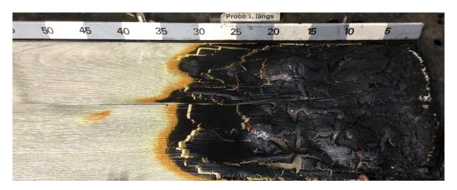
**5.2.** Reaction to fire sample 1 cross production direction
